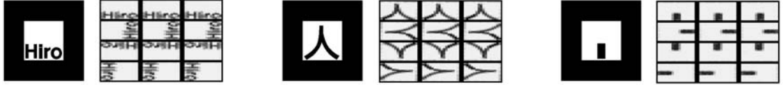
Figure 5: ARToolkit markers and their corresponding pattern files. (Left to right); 1) the Hiro marker image, 2) the pattern file patt.hiro , 3) the Kanji marker image, 4) the pattern file patt.kanji , 5) the Sample1 marker image, and 6) the pattern file patt.sample1 .
