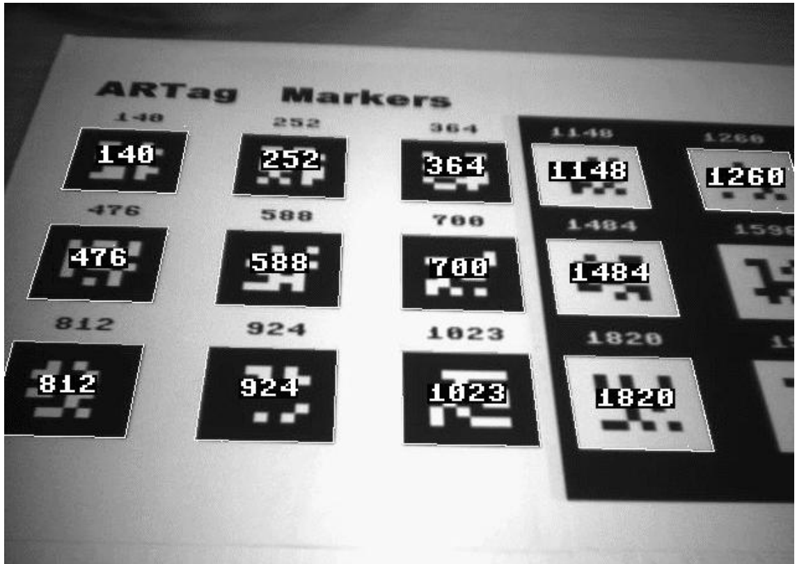
Figure 1: Markers detected in an image. Overlaid white border and ID number show automatic detection.
